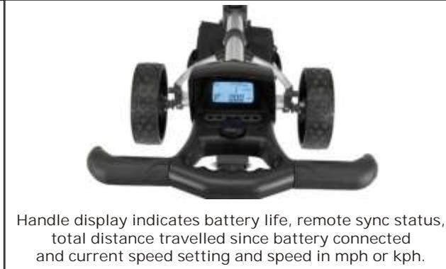
Handle display indicates battery life, remote sync status, total distance travelled since battery connected and current speed setting and speed in mph or kph.
